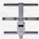
Elevatoe overload measurement
